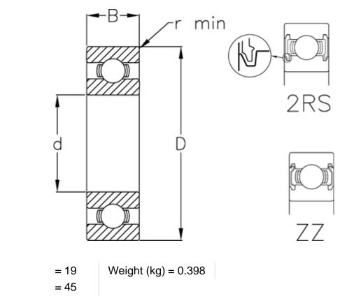
d = 45D = 85Dynamic load C (kN) = 32.5Max rpm greased = 7800Max rpm oil lubricated = 9200r min = 1.1Static load C0 (kN) = 20.4
